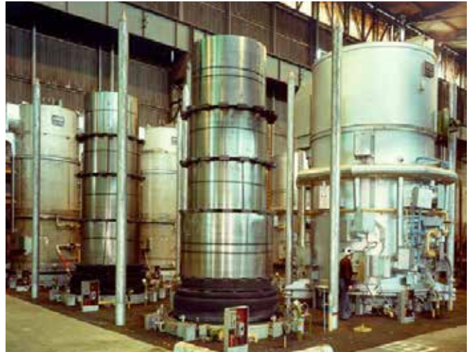
Figure 5. An 100% hydrogen bell annealing installation (photo courtesy of Ebner)
